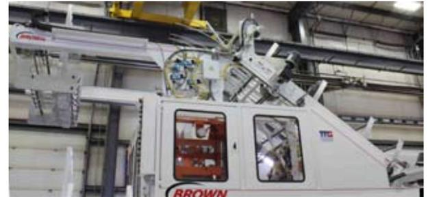
The sheet tamer/blower section provides control of the web loop for transition into the canopy treadle. This section is vital in automatic sheet threader mode. The formed web is automatically carried over the canopy and positioned into the feed cage to begin trimming and producing perfect parts on the very first cycle, minimizing scrap and set-up time.
