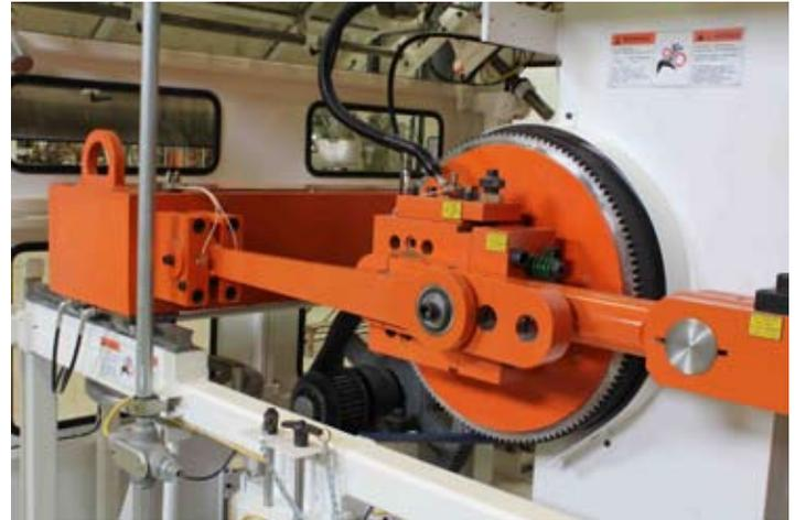
This system provides a significantly smoother trim press motion than traditional offerings that use counterweights attached to the main-shaft or fixed position counterbalance systems.
